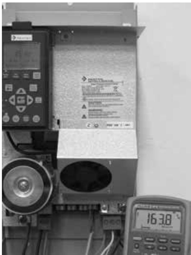
**Figure 18. 45Hz voltage measurement w/ LPF**
