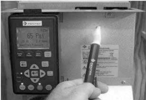
Figure 3. Easy ground check: Ungrounded
