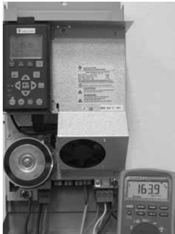
**Figure 21. 3 phase 45Hz voltage measurement**
