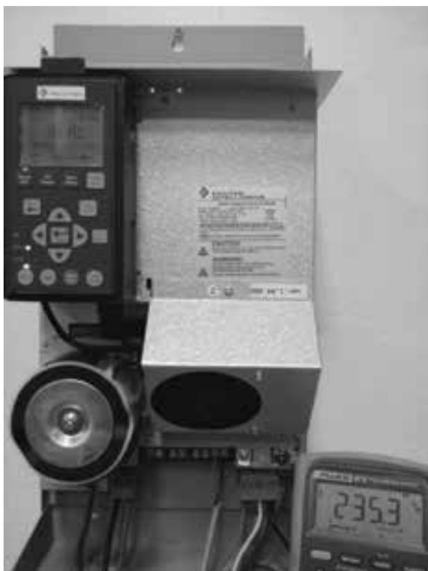
**Figure 22. 3 phase 60Hz voltage measurement**
